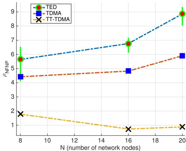
Fig. 8: Number of detected NFNPs,  $\rho_{\text{NFNP}}$  from (4), as a function of  $N$ . Vertical lines show the 5% and 95% ranges. Compared to TDMA and TT-TDMA, results show that using TED a significantly higher number of NFNPs can be detected.
