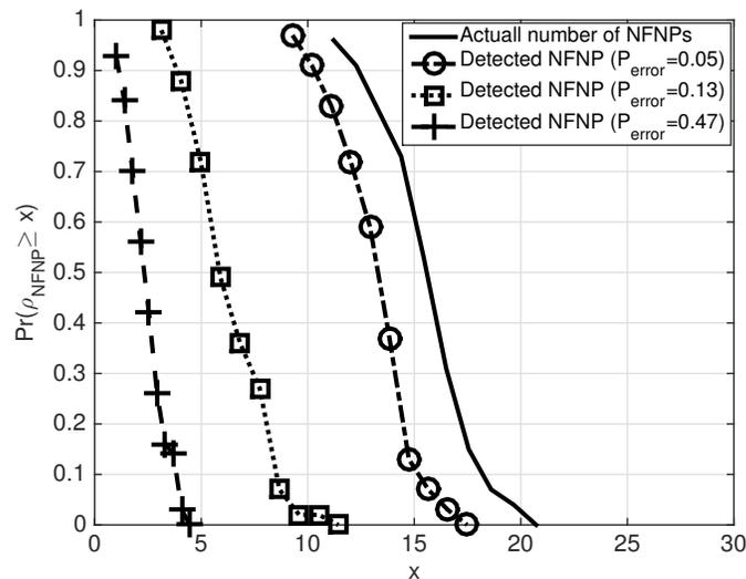
Fig. 9: C-CDF of the per-node number of detections of NFNPs,  $\rho_{\text{NFNP}}$  from (4), of TED. For a high packet error rate of 5%, misdetection is close to zero. Results show a high dependency of correct detections of NFNPs on the packet error rate.
