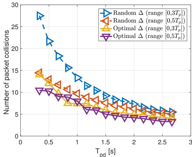
Fig. 5: Average number of packet collisions using the best of 500 random choices of  $\Delta$  and using  $\hat{\Delta}$  from (11) for two ranges of propagation delays. Propagation delays are chosen from a Rayleigh distribution. The figure shows a large benefit when using the calculated delay, especially for small networks
