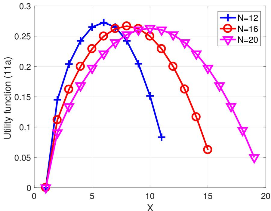
Fig. 3: Utility function (11a) as a function of the number of transmitting nodes  $X$  for three values of  $N$ . The figure shows that the optimal  $X$  is obtained for  $N/2$ .
