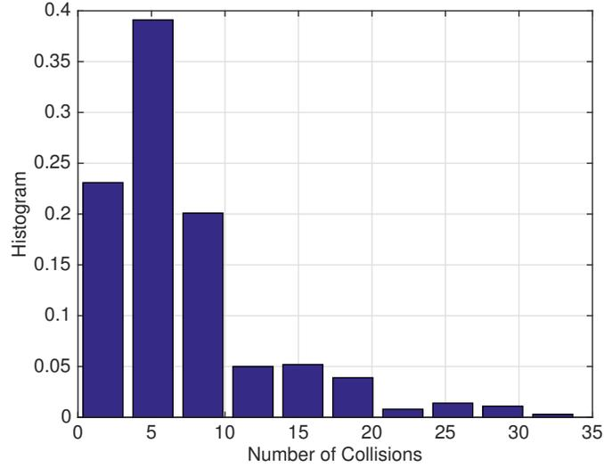
Fig. 2: Histogram of the number of collisions for randomized values of the delay vector  $\Delta$ . Since the number of collisions changes dramatically, we conclude that there is a strong dependence on the number of collisions on  $\Delta$ .
