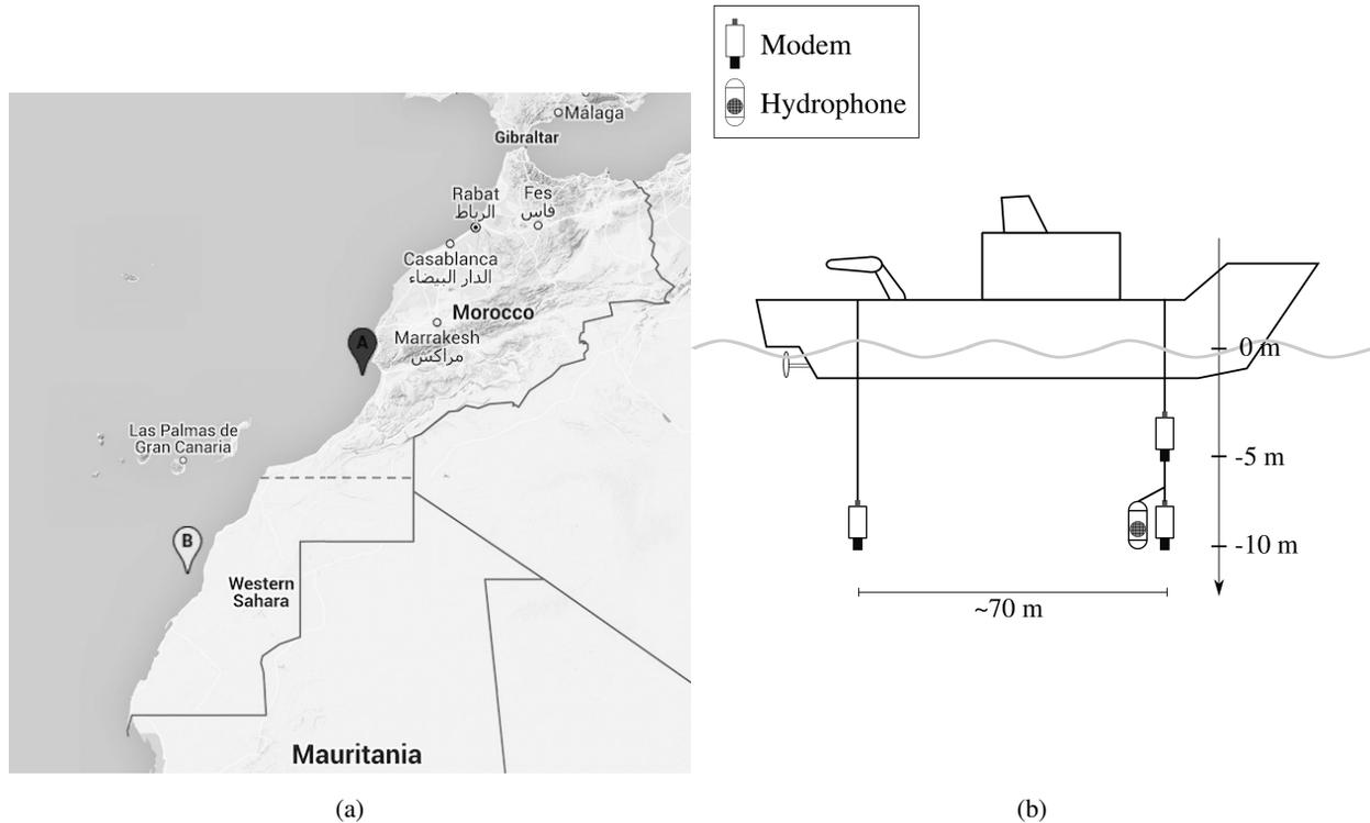
Fig. 10: Setup of sea experiment: (a) Locations where TED was tested during the ALOMEX'15 experiment, (b) Illustration of deployment setup.
