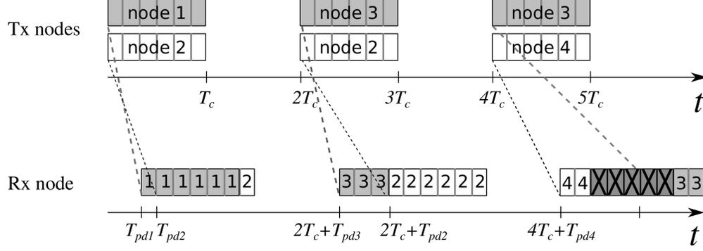
Fig. 4: Example for the detection of NFNPs. Nodes (2, 1) and (3, 2) are NFNPs, while nodes (3, 4) are not.
