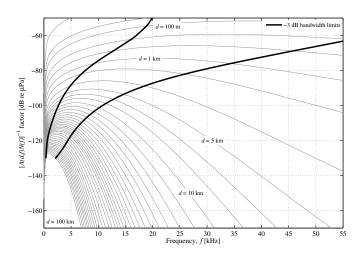
Fig. 1. Frequency-dependent part of the SNR for an acoustic tone transmitted underwater. Two black lines represent the lower and upper limit of the available transmit bandwidth B(d). Grey lines represent the  $[A(d,f)N(f)]^{-1}$  factor for different distances.
