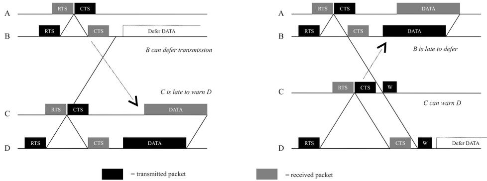
Figure 4. Scheme of transmissions in DACAP (adapted from [27]).
