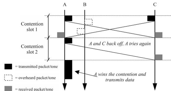
Figure 3. Scheme of transmissions in Tone-Lohi (adapted from [18]).
