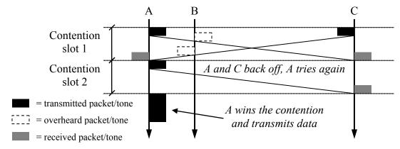
Fig. 1: An example of contention for channel access in T-Lohi.
