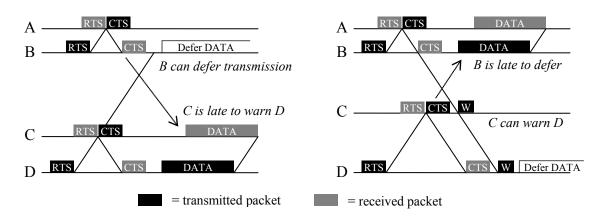
Fig. 2: Two situations where DACAP successfully avoids collisions.
