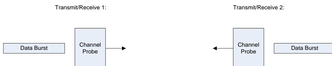
**Figure 2.6 Using a channel probe to extract information about the channel.**
