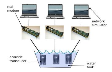
Fig. 2. Illustration of the TEST-BED setting: each modem is controlled by a single host (or a single NS instance).
