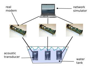
Fig. 1. Illustration of the EMULATION setting: a single host (or a single NS instance) controls multiple modems.
