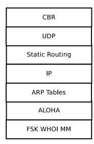
Fig. 4. Illustration of the protocol stack used during the feasibility tests.
