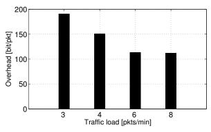
Fig. 5. Overhead for Uw-Polling as a function of the packet generation rate per node.
