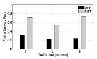
Fig. 6. PDR for MSUN as a function of the network packet generation rate.
