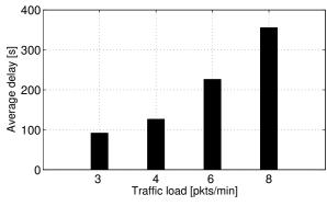
Fig. 4. Average delivery delay for Uw-Polling as a function of the packet generation rate per node.
