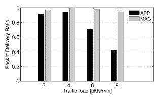
Fig. 3. Application-layer PDR for Uw-Polling as a function of the packet generation rate per node.
