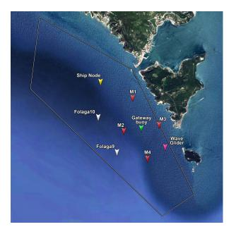
Fig. 1. A comprehensive snapshot of the network deployment during the CommsNet'13 sea trials in La Spezia, Italy. The external line delimits the operational area. The network includes bottom-mounted nodes, a ship node, an acoustic/radio gateway buoy, two autonomous underwater vehicles and one autonomous surface system. (Modified from a Google Maps screenshot.)
