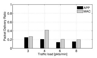
Fig. 9. PDR for U-Fetch as a function of the packet generation rate per node.
