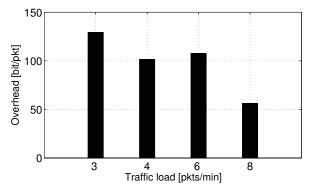
Fig. 11. Overhead for U-Fetch as a function of the packet generation rate per node.
