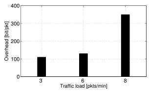
Fig. 8. Overhead for MSUN as a function of the network packet generation rate.
