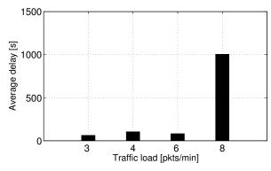
Fig. 10. Average delivery delay for U-Fetch as a function of the packet generation rate per node.
