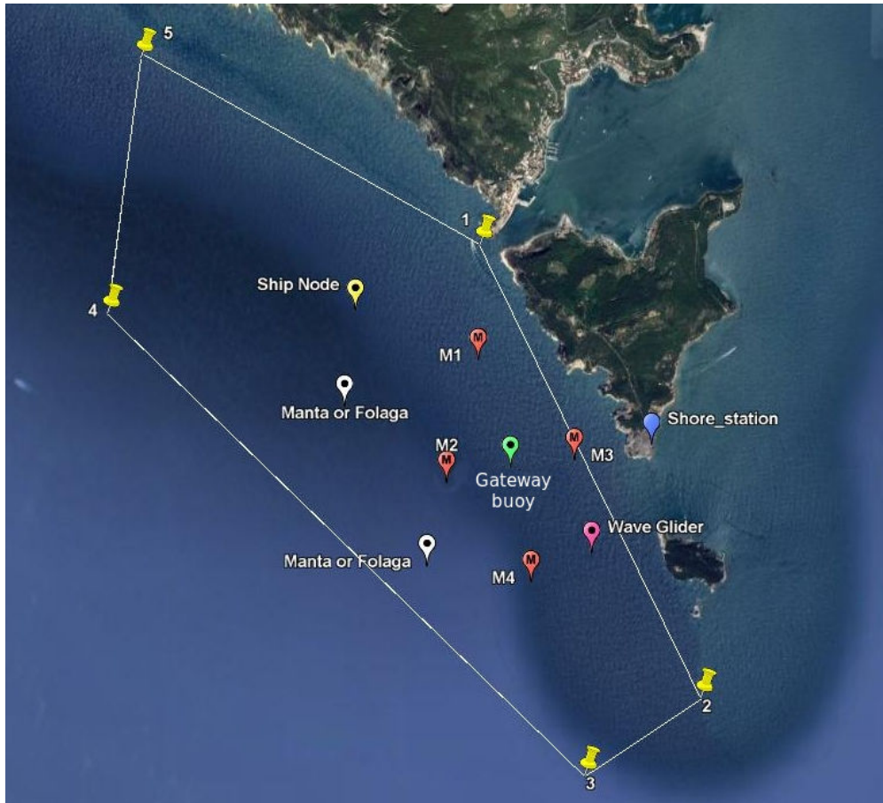
Figure 4. Typical topology of a complete network deployment during the CommsNet13 campaign carried out in La Spezia, Italy, in September 2013. The yellow pins denote the operational area. Nodes M1–M4 are bottom mounted nodes forming the so-called Littoral Ocean Observatory Network (LOON). The gateway buoy is a moored node mounting an acoustic modem and accessible via a radio interface. The wave glider is an autonomous system which harvests wave energy for propulsion. Folagas are GraalTech’s low-cost, torpedo-shaped AUVs. Mantas are University of Porto’s portable acoustic/radio gateway nodes. The ship node is in fact also a Manta, connected to an underwater modem hanging off the RV Alliance. (Best viewed in color.)
