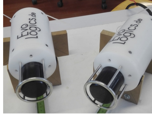
Figure 2: Setup of the FEC experiment in air in Scenario 1. The signals experienced little if any multipath propagation.
