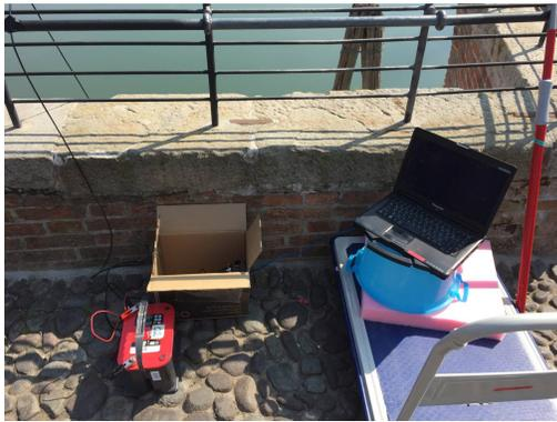
Fig. 1. Tests setup: box containing the boards, feeding batteries (left, red-colored) and control laptop (right)
