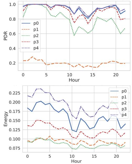
Fig. 10. Simulations of AMC PDR and energy performance: p1-p4 are fixed data rates (with p4 most robust), while p0 uses dynamic switching. [12]
