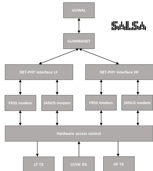
Fig. 5. SALSA software-defined modem architecture indicating the separate processes for the application layer (GUWAL), the network layer (GUWMANET), the low-frequency (LF) and high-frequency (HF) bands, and the FRSS-SALSA and JANUS modulations.
