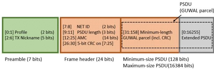
Fig. 6. Bit allocation for the coded preamble (green) and frame header with minimum-length packet size (orange) and with extended-length packet size (orange-gray). The “TX nickname” was included in the preamble to identify bad links.
