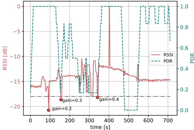
Fig. 4. PDR values obtained by switching the transmission gain based on an RSSI threshold.
