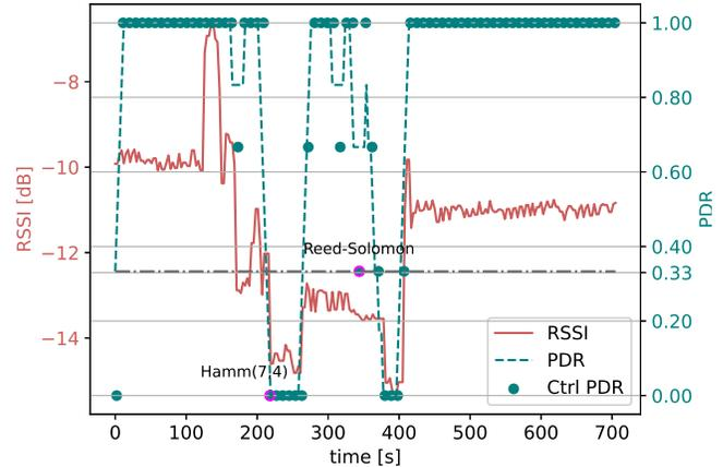
Fig. 7. PDR values obtained by switching the FEC scheme based on a PDR threshold.
