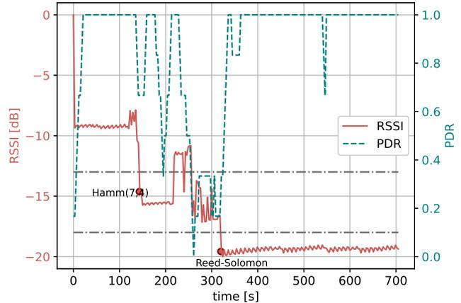
Fig. 5. PDR values obtained by switching the FEC scheme based on an RSSI threshold.
