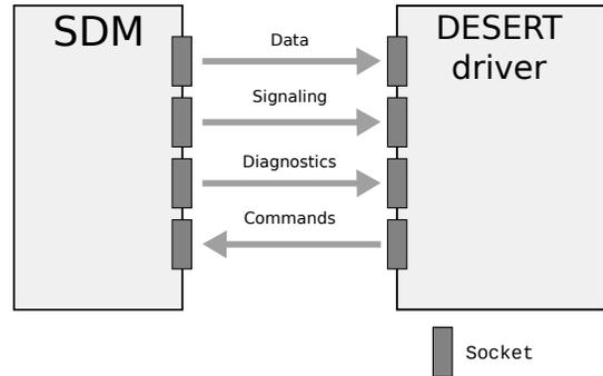
Fig. 2. Socket connections for Driver/SDM interaction.
