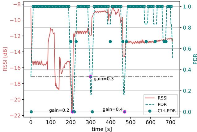
Fig. 6. PDR values obtained by switching the transmission gain based on a PDR threshold.
