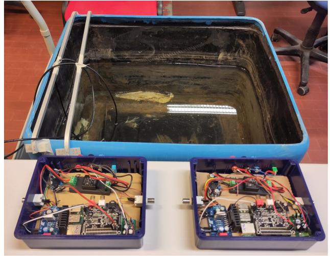
Fig. 3. Demo setup: the two SDM modems, on the table, in front of the water tank deployed during the test.
