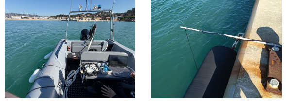
Fig. 3: Node RX deployed from a work boat (left) and Node TX deployed from a pier (right).
